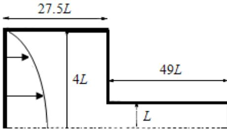
Figure 1: Schematic of 4:1 shape contraction flow.
