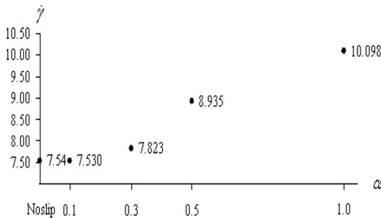
**Figure 9:** The peak of  $\dot{\gamma}$  versus  $\alpha$  on top downstream wall of Oldroyd-B fluid at  $We = 0.25$ .
