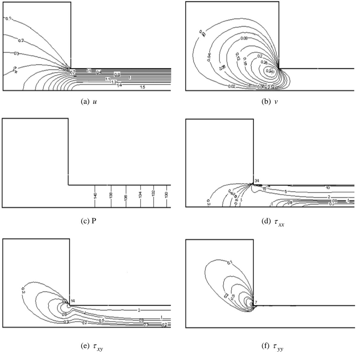
**Figure 13:** Line contour with slip along top downstream wall of Oldroyd-B fluid at  $\alpha = 0.1$ ,  $\Pi = 3.3$  and  $We = 1.0$ .
