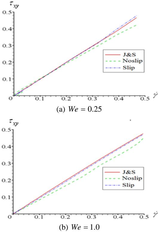
**Figure 11:** The comparison of  $\tau_{xy}$  versus  $\dot{\gamma}$  with J&S on top downstream wall of Oldroyd-B fluid.
