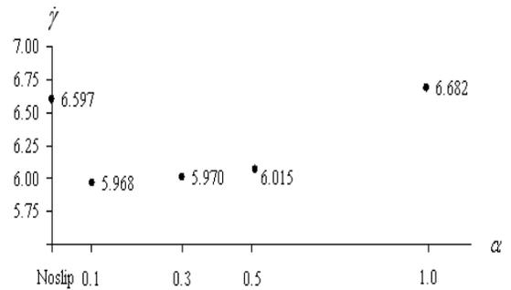
**Figure 5:** The peak of  $\dot{\gamma}$  versus  $\alpha$  on top downstream wall of Newtonian fluid at  $II = 2.3$ .
