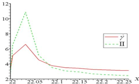
**Figure 3:** II and  $\dot{\gamma}$  along top downstream wall with no slip of Newtonian fluid.
