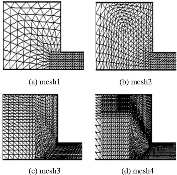
Figure 2: Sharp mesh pattern of 4:1 contraction flow.
