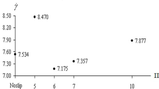
**Figure 10:** The peak of  $\dot{\gamma}$  versus  $II_{crit}$  on top downstream wall of Oldroyd-B fluid at  $We = 0.25$ .
