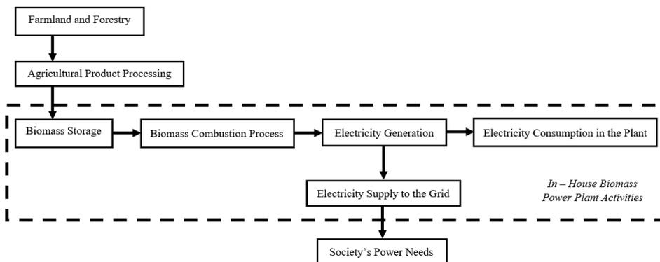
**Figure 3:** A general concept of biomass-based power plant operations.
