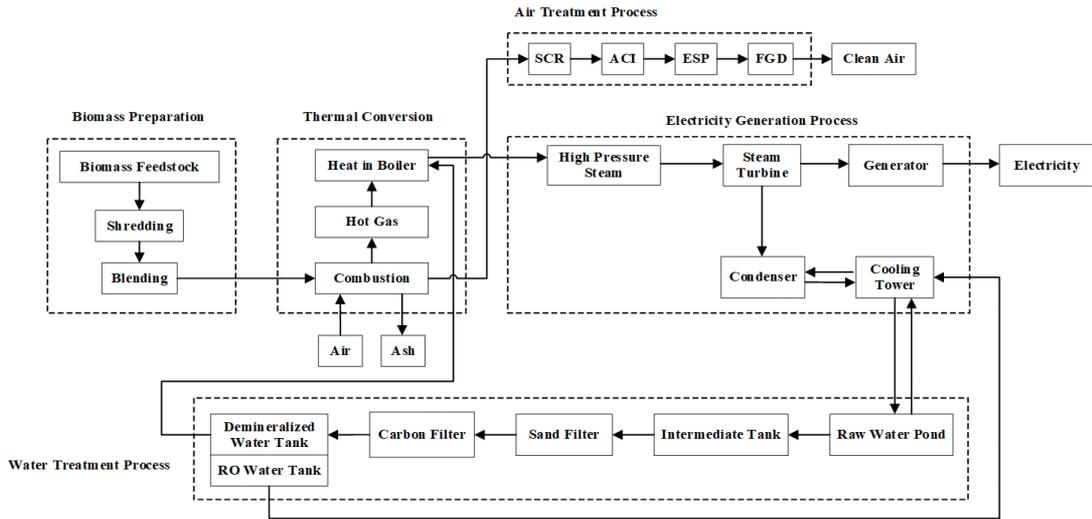
**Figure 6:** Environmental protection systems of the biomass power plant.
