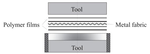
**Figure 2:** Schematic drawing of the cylindrical tool and a single reinforcement layer laminate build up.
