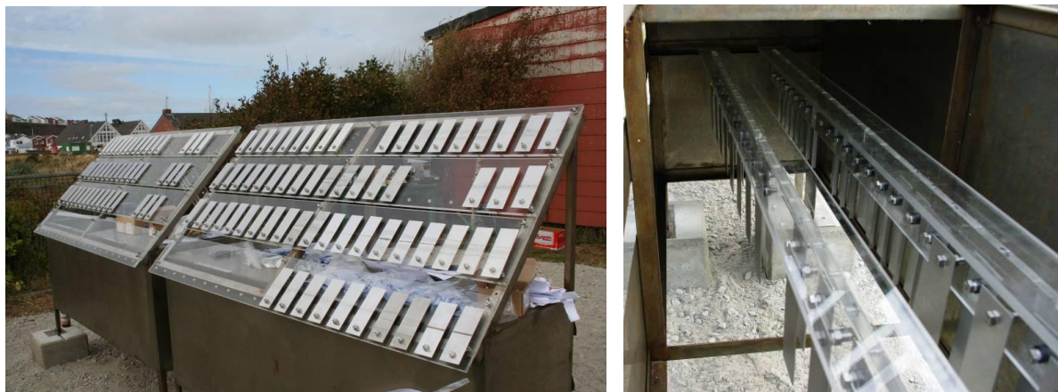
Figure 12: Rack with coupons on Helgoland
