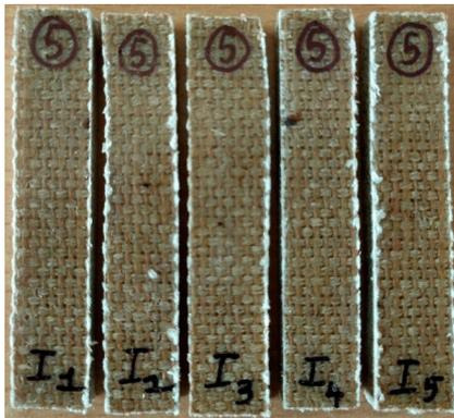
Figure 4: Sample specimen used in impact test.
