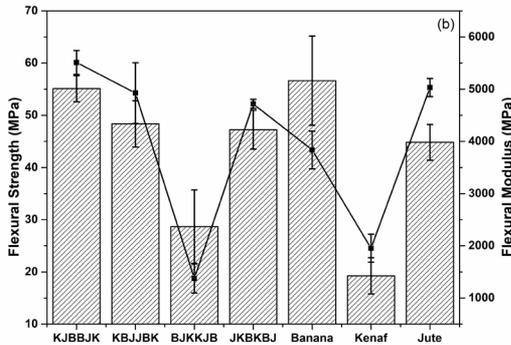
**Figure 9:** Flexural properties of investigated composites with individual fibres and various stacking sequences in the hybrid configuration.
