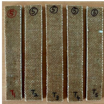
**Figure 2:** Sample specimen used in tensile test.
