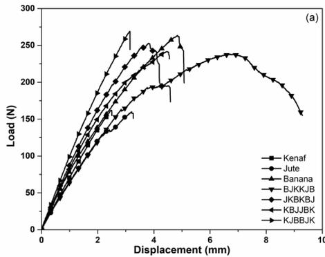
**Figure 8:** Flexural load vs. Displacement of investigated composites with individual fibres and various stacking sequences in the hybrid configuration.
