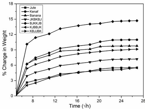
**Figure 11:** Moisture absorption characteristics of the investigated composites with individual fibres and various stacking sequences in the hybrid configuration.
