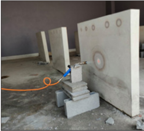
Figure 5: Fire behavior testing.
