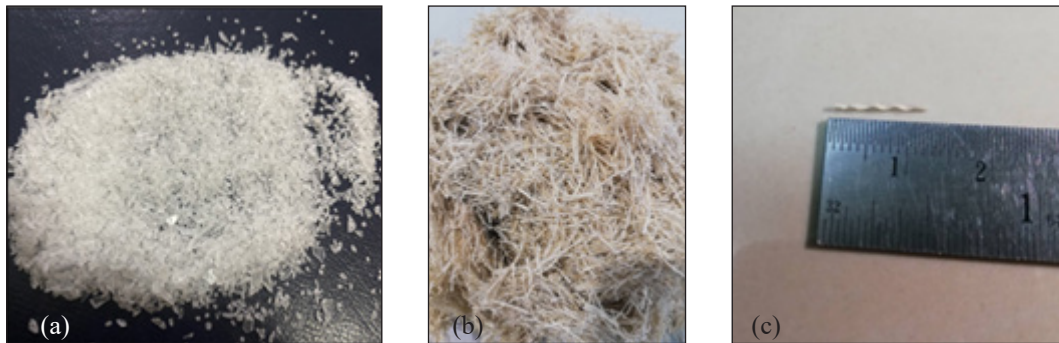
Figure 1: Plastic and agricultural wastes used in this study (a) PS (b) hemp fiber (c) 12 mm hemp fiber.
