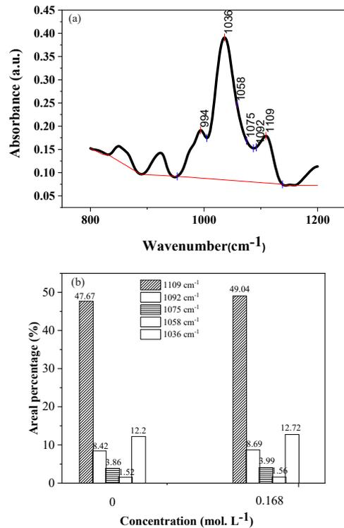
**Figure 6:** (a) IR spectrum used to compute the areal percentage of the significant peaks for the lithium-glycerol electrolyte ( $C = 0.168 \text{ mol. L}^{-1}$ ), (b) Areal percentages in the frequency region  $1100\text{--}800 \text{ cm}^{-1}$ .
