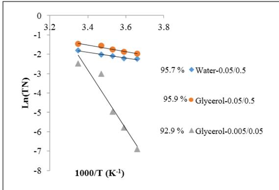
**Figure 8:** Arrhenius plots of transport number data of concentration cells 0.005/0.05 and 0.05/0.5 using power law in glycerol (Gly.); A comparison to water (Wat.)
