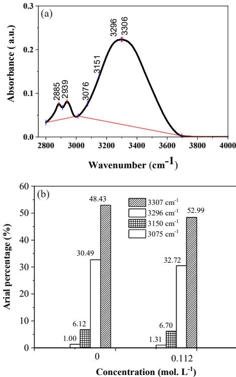
**Figure 4:** (a) IR spectrum used to compute the areal percentage of the significant peaks for the lithium-glycerol electrolyte (b) Areal percentages ( $C = 0.112 \text{ mol. L}^{-1}$ ) in the frequency region  $4000\text{--}2800 \text{ cm}^{-1}$ .
