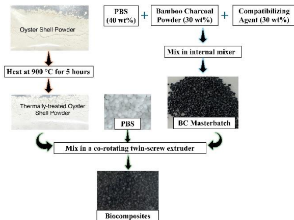
Figure 2: Diagram of BC-TSW-PBS composite preparation.
