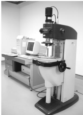
Fig. 1. Roundness measuring instrument, Talyrond 73.
