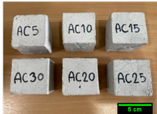
Figure 4 The obtained bricks from rice-husk ash mixed with cement.
